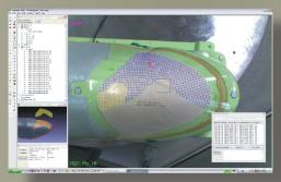
Allows deviation measurements
